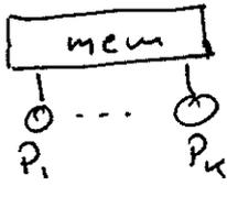
all processors can access every memory location simultaneously and in unit time
