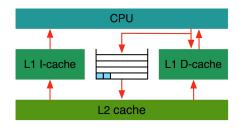
Reads can bypass previous writes for faster completion If read and write access different locations No order between write and following read (W ∠ R) W(a.1) W(b,1) R(a):0 write buffer R(b):0 2 b == 04 a==0 not seq. consistent
