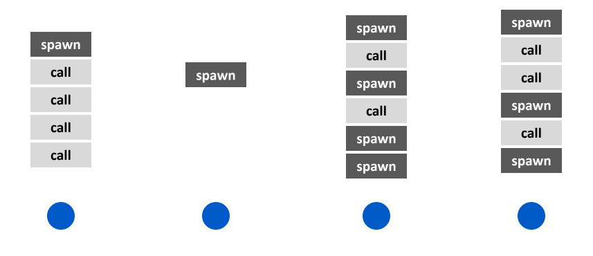
Each processor maintains a "ready deque:" deque of threads ready for execution; bottom is manipulated as a stack
