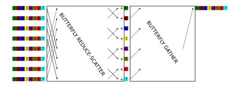
$$T_{\text{reduce}} = T_{\text{reduce-scatter}} + T_{\text{gather}}$$
