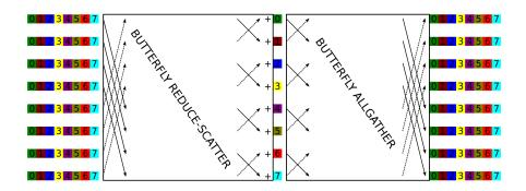
$$T_{\text{allreduce}} = T_{\text{reduce-scatter}} + T_{\text{allgather}}$$
