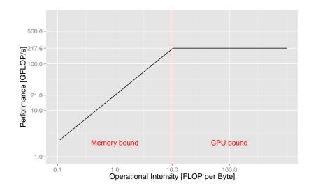
If a measurement result lies on the left side of the diagram and on the roofline (drawn in black) it is bound by memory bandwidth. If it lies on the right side of the roofline it is bound by computational bandwidth. If it lies below the roofline, it is bound by something else i.e., integer performance, which is not represented in the (simple) roofline model.
